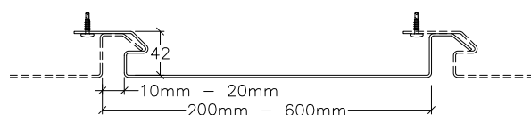
Slimwall SFP42-S ; module 200mm to 600mm
