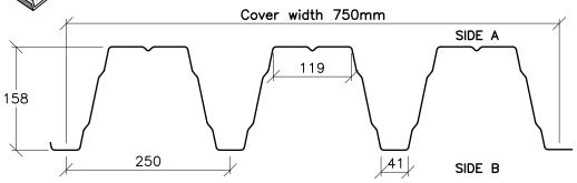
Available as web or fully perforated - refer to APL for load/span information
